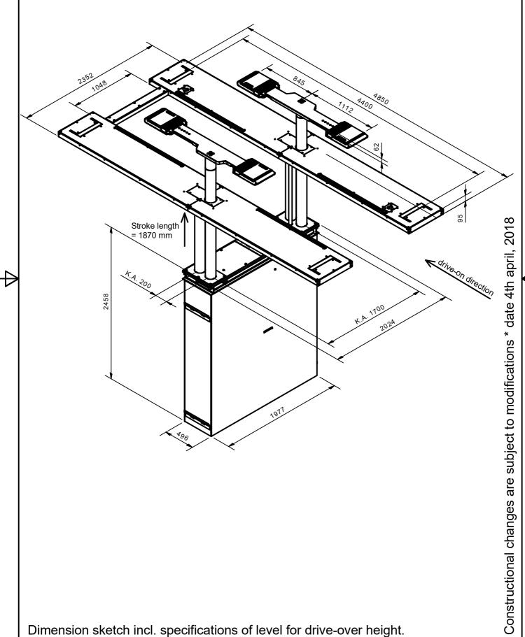
Dimension sketch incl. specifications of level for drive-over height.
