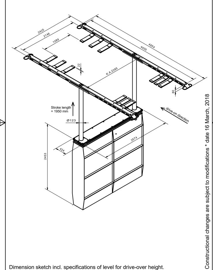
Dimension sketch incl. specifications of level for drive-over height.
