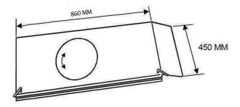
The plate has a maximum load of 1250 kg (axle load of 2500 kg). The plate can move 40 mm in all directions. The height is 40 mm. The turn table can rotate 360°. The plates are supplied in pairs.
