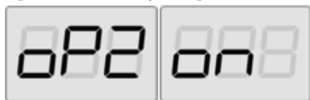
Fig. 30: Enabling operator 2 memory Operator 1 memory is kept
