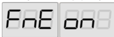
Fig. 28: Enabling imbalance display in high resolution
