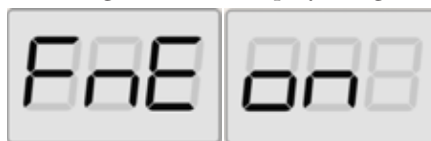
Fig. 28: Enabling imbalance display in high resolution
