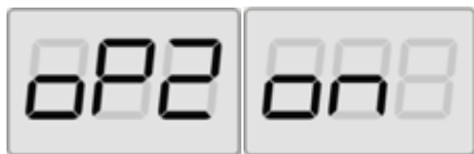
Fig. 30: Enabling operator 2 memory Operator 1 memory is kept
