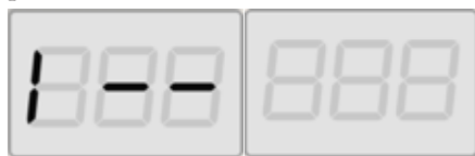
Fig. 24: Search for the balancing planes: the left display indicates to move the sensor back (move it to the left) to find the exact internal position of the balancing planes
