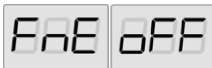
Fig. 29: Disabling imbalance display in high resolution
