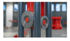
safety. The **obstruction system** stops the lift automatically when touching down on an obstacle.
